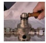
All pressure reducers are tested before being packaged; during test they are pre-set at the outlet pressure of 3 bars; outlet pressure can be easely adjusted once the pressure reducing valve in installed on site.
